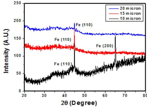
Fig.3: XRD of TiSiBC film for 10µm, 15µm and 20µm coating
