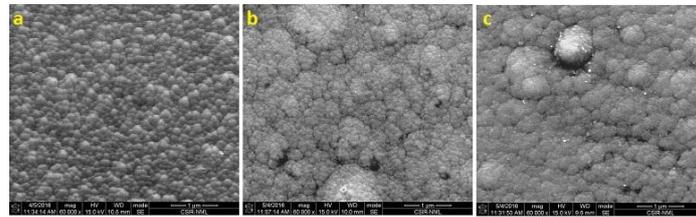
Fig.4: SEM micrographs of as deposited TiSiBC film for a) 10µm, b) 15µm and c) 20µm coating thickness
