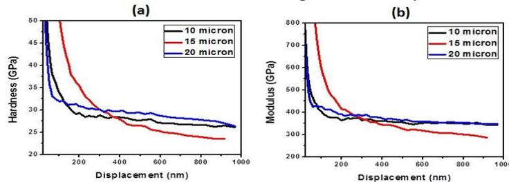
**Fig.6:** a) Displacement Vs Hardness and b) Displacement Vs Modulus graph for TiSiBC coated samples at different thickness
